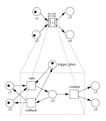
Figure 17: The low-level behavior of a task.
