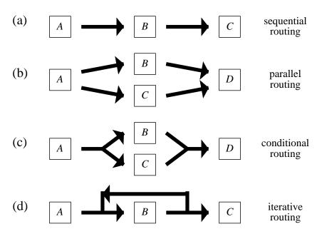
Figure 3: Four routing constructs.
